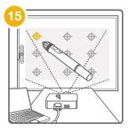
Launch the eBeam software, calibrate the system.
