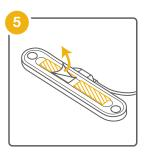
Peel the Command Adhesive backing from the receiver.
