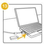
Connect the wireless adapter to the USB port.
