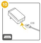
Connect the eBeam USB cable to the power supply.
